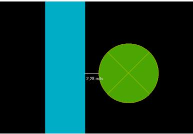
Check for to less distence between solder mask and drill or SMD pads.
