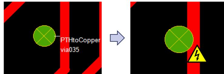
For un-plated drills, the distance is needed for tenting the hole during the plating process to avoid copper in the hole. When the un-plated drill could not be securely tented, a second drill process after the plating process is needed instead.
